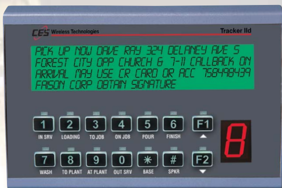
TRK-240 mobile display terminal with the GPS receiver option.
